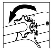
If the gas block arrow indicates you are on the suppressed (1-dot) setting, then you can only rotate counterclockwise to increase gas flow. (shown left)
