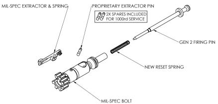
The procedure to field strip your bolt carrier group does not change with the addition of the Gen 2 firing pin & reset spring. The Gen 2 firing pin features a retaining boss which should hold the reset spring in place during assembly and disassembly.
