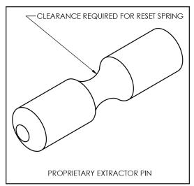
The Gen 2 firing pin & reset spring use a proprietary extractor pin. You cannot use a mil-spec extractor pin with the reset spring..
