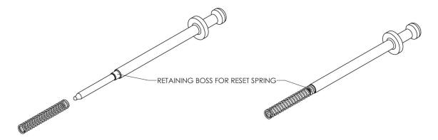
If the reset spring has slipped off this boss during operation then tap the tail of the bolt on a hard surface to bring the reset spring rearward, and use the tip of the firing pin, or a small pick if available, to fish out the spring.
