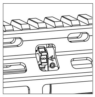
SUPPRESSED (1-DOT) - This setting has the smallest gas port, which restricts the gas as much as possible, for when you're running a silencer with high back pressure.
