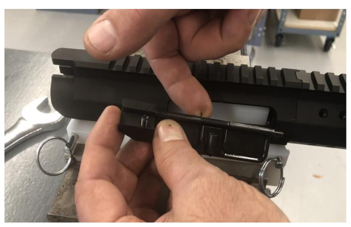
Next: Slide the pin into the hole in the Upper Receiver as shown below. Maintain pressure on the small leg of the Dust Cover Spring, it will rest against the upper receiver, keeping pressure on the Dust Cover Spring.
