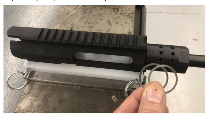
There are (2) thicknesses of shims included, try one shim at a time until you get the correct torque settings.
