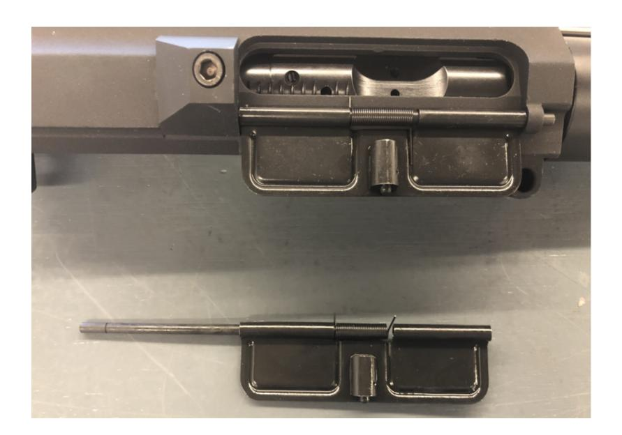
The long leg of the spring is towards the front of the upper. Now take the long leg of the spring and rotate it, and rest it against the dust cover (see picture on next page).
