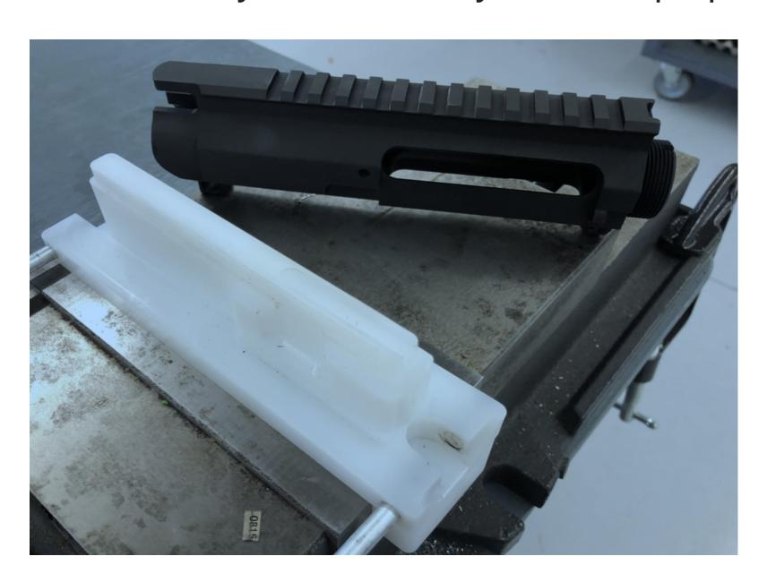
Mount Upper receiver in the fixture, insert locking pins. Apply anti-seize compound to the external thread on The Upper receiver (shown below).
