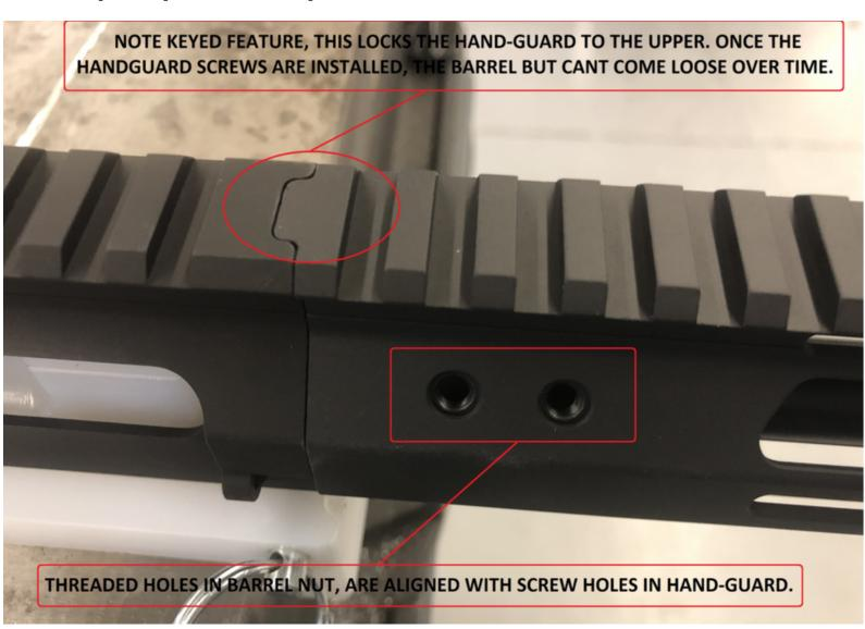
NOTE: Apply Loctite to the 10-32 Button Head screws.
