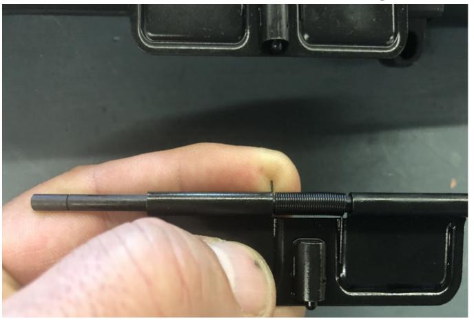
Next: Slide the Dust Cover Pin, into the Case Deflector as shown below.
